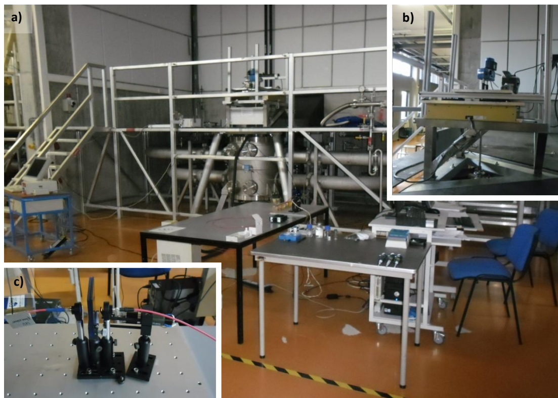
Figure 3.5 Pictures from total experimental setup 3 (a), with magnifications of the rotation part with extension tube 1 (b) and the optical part outside the magnet (c). In c), light from a halogen light source passes a shutter and filters after which it is coupled into a fiber again which goes into the magnet and is mounted on the insert. More pictures are shown in supplemental material S4.
