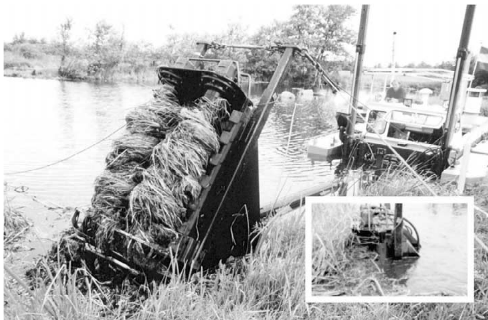
Figure 8. The 'Kraggenvreter' ('Scragh Wolf'), a floating device developed by the State Forestry Service to create new peat holes in fen peatlands. Peat including its vegetation is removed by the machine's harvester arm, mixed with water and piped to a depot. Inlay: the wolf's head (harvester arm) busy under water. Photo: L. Brouwer, State Forestry Department De Weerribben.
