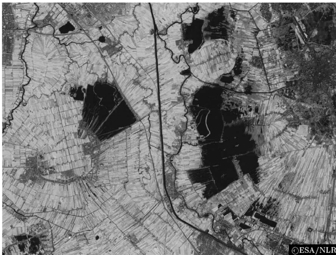
Figure 2. A satellite image of a fen area near Utrecht clearly shows the rectilinear method of peat extraction, which is characteristic for most Dutch fens. The destruction of peat baulks, mostly by storms, resulted in shallow lakes (dark) like the Vinkeveense Plassen (left) and Loosdrechtse Plassen (right). European Space Agency (ESA) / National Aerospace Laboratory (NLR). Scale 1:155 000.
