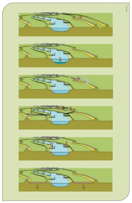
Figure 6 Alternatives to dike heightening are, from top to bottom, setting back dikes, deepening low flow channel, detention reservoirs, removal of hydraulic bottle necks, lowering groynes, and lowering floodplains.
