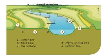
Figure 3 Two-tier dike structures and groynes for flood protection along the rivers in The Netherlands.
