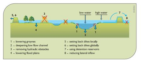
Figure 5 Alternatives to dike heightening for increasing flood flow capacity of rivers.
